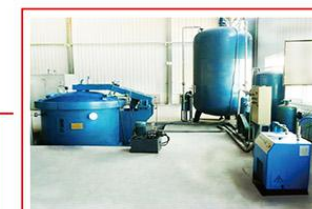
VPI impregnation equipment
