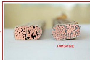
Varnish filling amount anatomical physical map. Faraday used the imported insulation material to insure that generator mechanical and electrical insulation at the highest level
